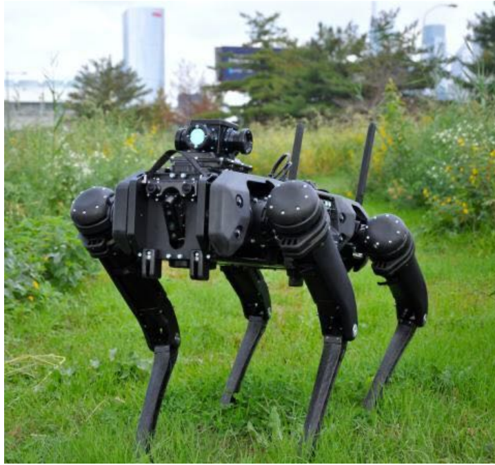
A video camera or sensor package (known as a “payload”) can be attached to a robot dog. Photo: Courtesy Ghost Robotics.
